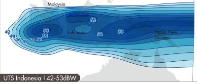
Ku-Band Transponders: 51 (49 x 54 MHz and 2 x 108 MHz) Polarization: Linear (H&V)
