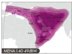
Ka-Band Transponders: 6 (out of 4 x 435 MHz &  $4 \times 225$  MHz)
