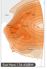
C-Band Transponders: 32 (8 x 36 MHz, 22 x 72 MHz & 2 x 104 MHz) Polarization: Linear (H&V)
