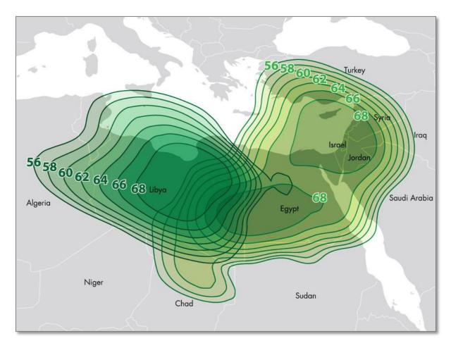
ABS-4 | West Beam | 56-68dBW ABS-4 | East Beam | 56-68dBW
