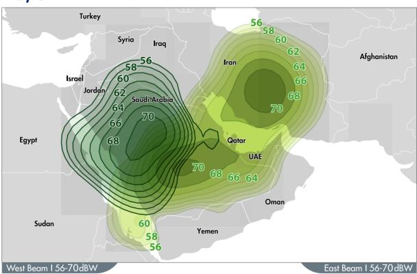
Ku/S-band Transponders: 2 x 25MHz Polarization: Linear / Circular Uplink/Downlink Frequency: 13.858 – 13.883 / 2.630 – 2.655
