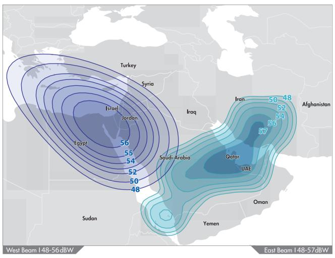
Ku/Ku Band Transponders: 2 x 25MHz Polarization: Linear / Linear Uplink/Downlink Frequency: 13.824 – 13.849 / 12.214 – 12.239
