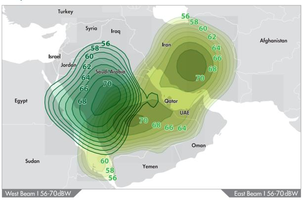
Ku/S Band Transponders:  $2\times25$ MHz Polarization: Linear / Circular Uplink/Downlink Frequency: 13.858-13.883/2.630-2.655
